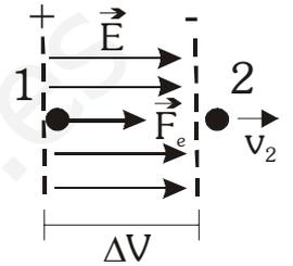
$$E_M = cte \rightarrow \Delta E_c = -E_{p_e} \rightarrow \frac{1}{2}mv_2^2 - 0 = -q \cdot (V_2 - V_1) \rightarrow \frac{1}{2}mv_2^2 = |q \cdot \Delta V|$$
