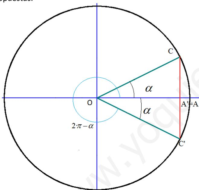
$$\left\{ \begin{array}{l} \text{sen } (2\pi - \alpha) = \frac{\overline{A'C'}}{\text{radio}} = \frac{-\overline{AC}}{\text{radio}} = -\text{sen } \alpha \\ \text{cos } (2\pi - \alpha) = \frac{\overline{OA'}}{\text{radio}} = \frac{\overline{OA}}{\text{radio}} = \text{cos } \alpha \\ \text{tg } (2\pi - \alpha) = \frac{\text{sen } (2\pi - \alpha)}{\text{cos } (2\pi - \alpha)} = \frac{-\text{sen } \alpha}{\text{cos } \alpha} = -\text{tg } \alpha \end{array} \right.$$
