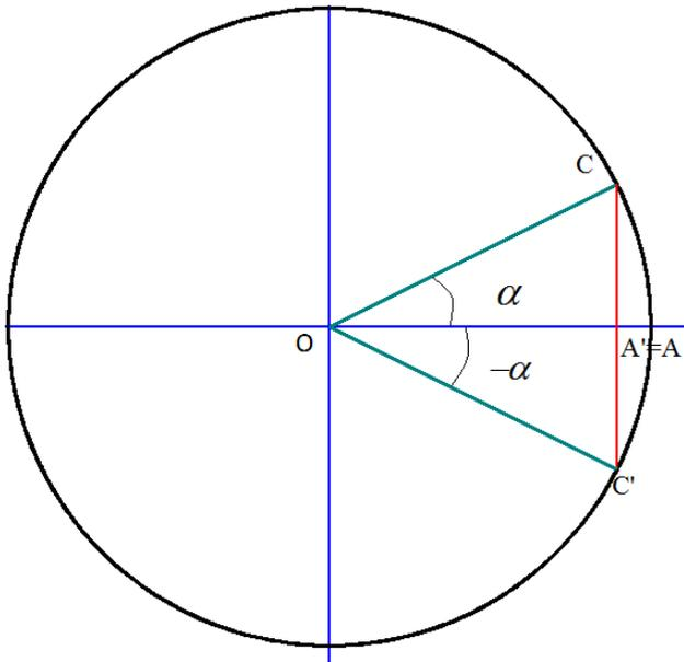
$$\begin{cases} \operatorname{sen}(-\alpha) = \frac{\overline{A'C'}}{\text{radio}} = \frac{-\overline{AC}}{\text{radio}} = -\operatorname{sen} \alpha \\ \operatorname{cos}(-\alpha) = \frac{\overline{OA'}}{\text{radio}} = \frac{\overline{OA}}{\text{radio}} = \operatorname{cos} \alpha \\ \operatorname{tg}(-\alpha) = \frac{\operatorname{sen}(-\alpha)}{\operatorname{cos}(-\alpha)} = \frac{-\operatorname{sen} \alpha}{\operatorname{cos} \alpha} = -\operatorname{tg} \alpha \end{cases}$$
