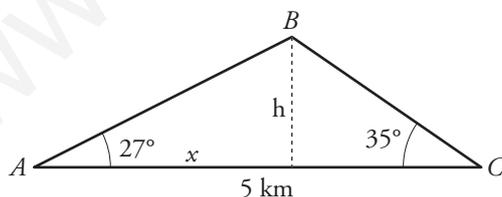
$$\left. \begin{aligned} \operatorname{tg} 27^\circ &= \frac{h}{x} \\ \operatorname{tg} 35^\circ &= \frac{h}{5 - x} \end{aligned} \right\} \left. \begin{aligned} h &= x \operatorname{tg} 27^\circ \\ h &= (5 - x) \operatorname{tg} 35^\circ \end{aligned} \right\}$$
