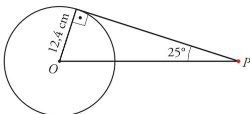
$$\begin{aligned} \operatorname{sen} 25^\circ &= \frac{12,4}{PO} \rightarrow \\ \rightarrow PO &= \frac{12,4}{\operatorname{sen} 25^\circ} \approx 29,34 \text{ cm} \end{aligned}$$
