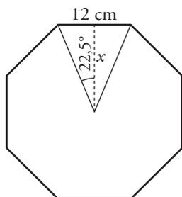
$$\frac{360^\circ}{8} = 45^\circ; \frac{45^\circ}{2} = 22,5^\circ; \text{apotema: } x$$
