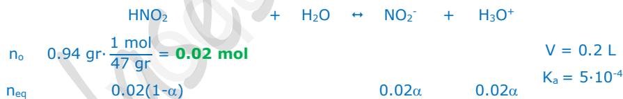
$$K_a = \frac{[\text{NO}_2^-]_{\text{eq}} \cdot [\text{H}_3\text{O}^+]_{\text{eq}}}{[\text{HNO}_2]_{\text{eq}}} \rightarrow 5 \cdot 10^{-5} = \frac{\left(\frac{0.02\alpha}{0.2}\right)^2}{\frac{0.02(1-\alpha)}{0.2}} \rightarrow -2 \cdot 10^{-3}\alpha - 10^{-6}\alpha + 10^{-6} = 0 \rightarrow \begin{cases} \alpha = -0.0226 \\ \alpha = \mathbf{0.0221} \end{cases} \rightarrow [\text{H}_3\text{O}^+]_{\text{eq}} = \mathbf{2.21 \cdot 10^{-3} \text{ M}}$$
