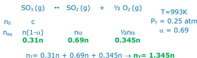
$$P_P = P_T \cdot \chi \rightarrow \begin{cases} P_{\text{SO}_3} = 0.25 \cdot \frac{0.31n}{1.345n} \rightarrow P_{\text{SO}_3} = 0.0576 \text{ atm} \\ P_{\text{SO}_2} = 0.25 \cdot \frac{0.69n}{1.345n} \rightarrow P_{\text{SO}_2} = 0.128 \text{ atm} \\ P_{\text{O}_2} = 0.25 \cdot \frac{0.345n}{1.345n} \rightarrow P_{\text{O}_2} = 0.0641 \text{ atm} \end{cases}$$
