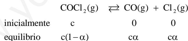
$$K_c = 0'083 = \frac{[\text{CO}] \cdot [\text{Cl}_2]}{[\text{COCl}_2]} = \frac{c\alpha^2}{(1 - \alpha)} = \frac{0'2\alpha^2}{(1 - \alpha)} \Rightarrow \alpha \approx 0'47 = 47\%$$
