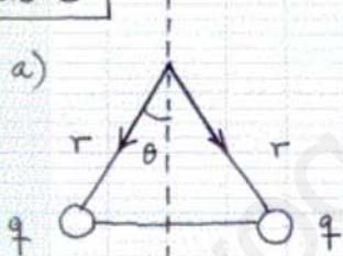
$$\begin{aligned} \vec{E} &= k \frac{|q|}{r^2} (-\sin\theta, -\cos\theta) + k \frac{|q|}{r^2} (\sin\theta, -\cos\theta) \\ &= k \frac{|q|}{r^2} (0, -2\cos\theta) \quad \text{amb } \theta = 30^\circ \end{aligned}$$
