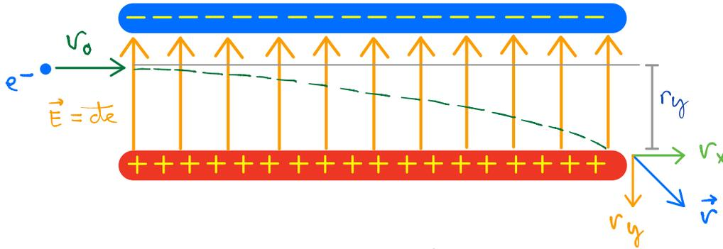
$$a) \vec{F} = q \cdot \vec{E} = m \cdot \vec{a} \Rightarrow \vec{a} = \frac{q \cdot \vec{E}}{m} = \frac{-1,6 \times 10^{-19} \times 10^5}{9,11 \times 10^{-31}} \approx -1,756310 \times 10^{16} \text{ m/s}^2 \approx -1,76 \cdot 10^{16} \text{ m/s}^2$$
