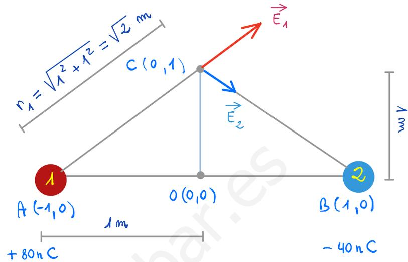
$$\vec{E}_1 = K \frac{Q_1}{r_1^2} \vec{u}_1 = 9 \cdot 10^9 \cdot \frac{80 \cdot 10^{-9}}{2} \left( \frac{1}{\sqrt{2}} \vec{i} + \frac{1}{\sqrt{2}} \vec{j} \right) \approx 254,6 \vec{i} + 254,6 \vec{j} \frac{\text{N}}{\text{C}}$$
