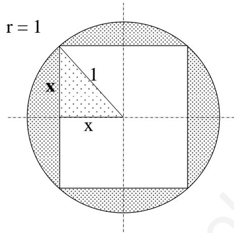
$$x^2 + x^2 = 1^2 \quad ; ; \quad 2x^2 = 1 \quad ; ; \quad x = \sqrt{\frac{1}{2}} = \frac{1}{\sqrt{2}} = \frac{\sqrt{2}}{2} \quad ; ; \quad \ell = 2x = \underline{\underline{\sqrt{2} = \ell}}$$
