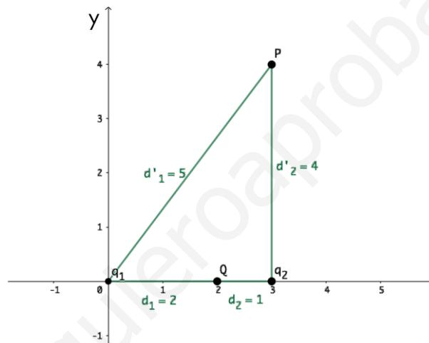
$$V(Q) = V_1(Q) + V_2(Q) = K \frac{q_1}{d_1} + K \frac{q_2}{d_2} = 9 \cdot 10^9 \frac{10 \cdot 10^{-6}}{2} + 9 \cdot 10^9 \frac{20 \cdot 10^{-6}}{1} = 2,25 \cdot 10^5 V$$
