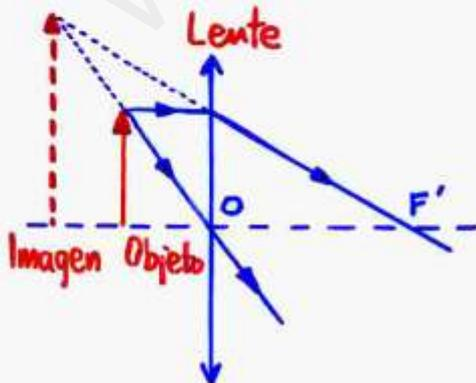
$$\left\{ \begin{array}{l} \frac{1}{f'} = \frac{1}{s'} - \frac{1}{s} \\ A = \frac{s'}{s} \end{array} \right. ; \left\{ \begin{array}{l} \frac{1}{0,10} = \frac{1}{s'} - \frac{1}{-0,05} \\ A = \frac{s'}{-0,05} \end{array} \right.$$
