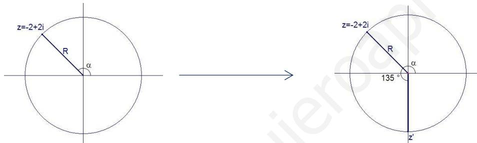
$$z = -2 + 2i \Rightarrow \begin{cases} R = \sqrt{(-2)^2 + 2^2} = \sqrt{8} = 2\sqrt{2} \\ \alpha = \operatorname{arctg}(-1) = 135^\circ, \text{ al ser } 90^\circ < \alpha < 180^\circ \end{cases} \Rightarrow z = 2\sqrt{2} e^{i 135^\circ}$$
