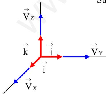
$$\vec{V}_x = V_x \cdot \vec{i} \quad , \quad \vec{V}_y = V_y \cdot \vec{j} \quad , \quad \vec{V}_z = V_z \cdot \vec{k}$$
