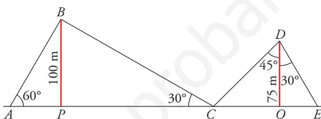
$$\operatorname{sen} 60^\circ = \frac{100}{\overline{AB}} \rightarrow \overline{AB} \approx 115,47 \text{ m} \quad \operatorname{tg} 60^\circ = \frac{100}{\overline{AP}} \rightarrow \overline{AP} \approx 57,74 \text{ m}$$
