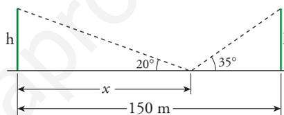
$$\left. \begin{aligned} h &= x \operatorname{tg} 20^\circ \\ h &= (150 - x) \operatorname{tg} 35^\circ \end{aligned} \right\} (150 - x) \operatorname{tg} 35^\circ = x \operatorname{tg} 20^\circ \rightarrow x = \frac{150 \cdot \operatorname{tg} 35^\circ}{\operatorname{tg} 20^\circ + \operatorname{tg} 35^\circ} = 98,7 \text{ m}$$
