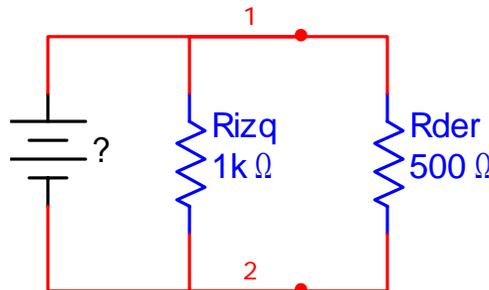
$$R_{total} = \frac{R_{der}R_{izq}}{R_{der} + R_{izq}} = \frac{1k * 500}{1k + 500} = 333.3\Omega$$
